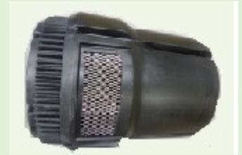
With a long-handled wire brush vigorously scour the Bio-drum™ screen. If the drum screen is severely encrusted with debris, it may be necessary to use a nail or screwdriver to clear the holes in the Bio-drum™ screen.
