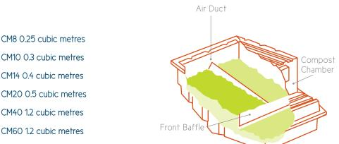
Once the woodshavings have been added, dampen down well with water (spray with a hose through the top inspection door). This breaks the surface tension and allows the bulking material to begin absorbing the urine that will enter the tank. If this is not done liquid can simply run off the organic material without slowly leaching through.
