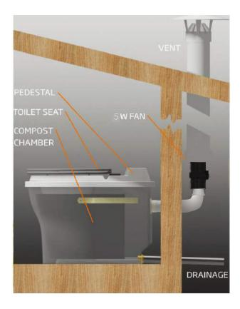
The NL2 uses the process of organic decomposition to break down waste into safe compost. Removal of the compost chambers is as easy as opening the toilet lid, removing the compost chamber and replacing it with an empty one.
